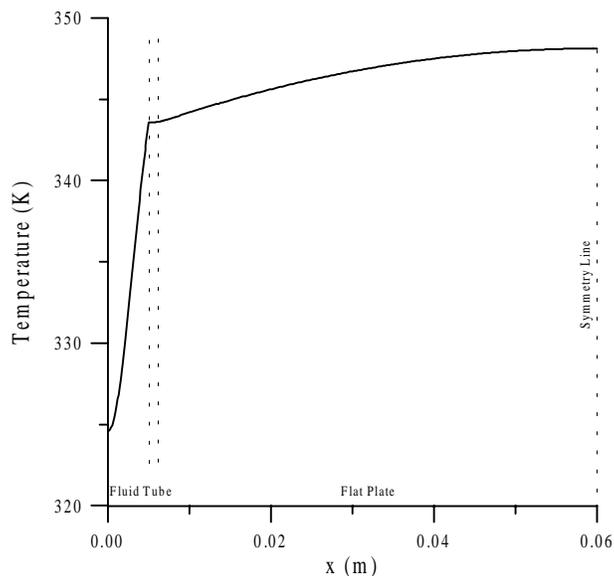
Figure 4: Temperature distribution in the cross-section of the collector.
