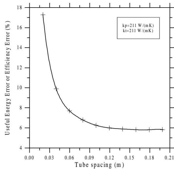
Figure 7: Useful energy gain and collector efficiency error variation with tube spacing.
