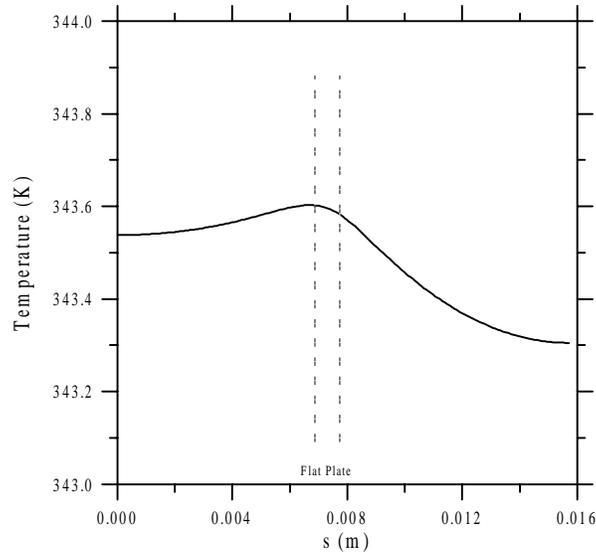
Figure 3: Temperature distribution in the tube internal wall surface.
