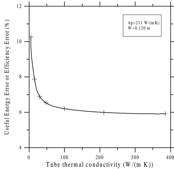
Figure 6: Useful energy gain and collector efficiency error variation with tube wall thermal conductivity.
