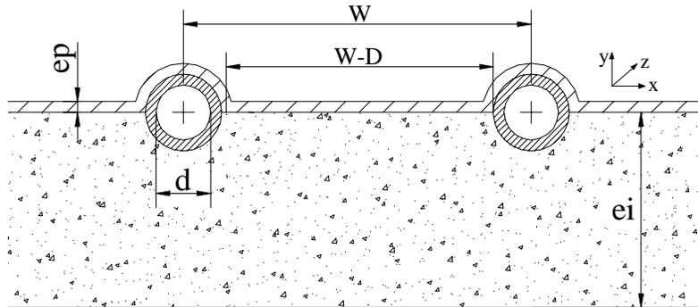
Figure 1: Cross-section of a basic flat plate solar collector.
