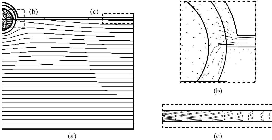
Figure 5: (a) Isothermal lines in the cross-section of the collector, (b) Two-dimensional heat flux in the tube, (c) Two-dimensional heat flux in the flat plate.
